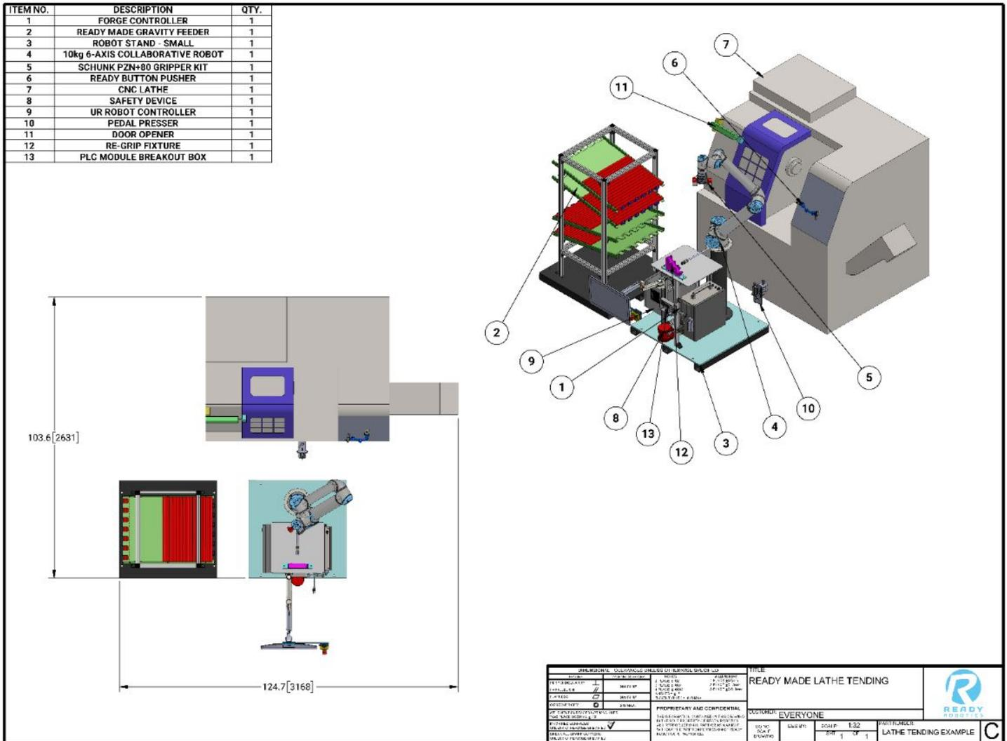
Figure 1 : READY Made Automated CNC lathe configuration with a collaborative robot
